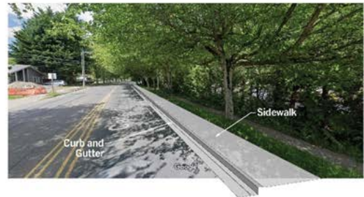
STREET VIEW RENDERING: NEW CURB AND SIDEWALK CONSTRUCTED IN EXISTING PARKING AREA
