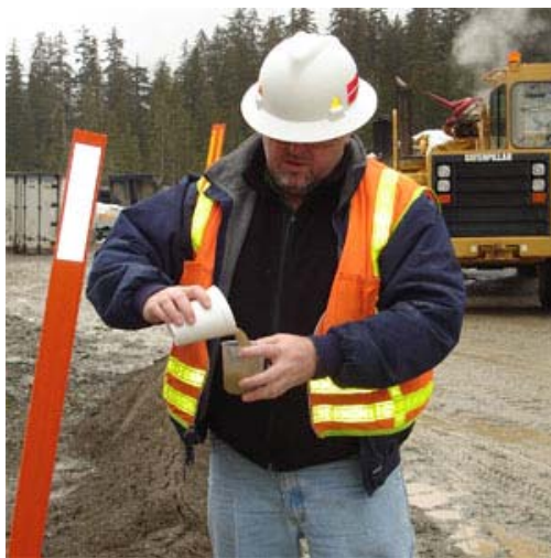
Collecting water for turbidity testing
